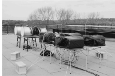
Fig. 2. Fourteen-element Bonner sphere spectrometer located on the roof of the IBM T.J. Watson Research Center. The suitcases and connector ends of the large detectors were covered in plastic bags to prevent water damage.
