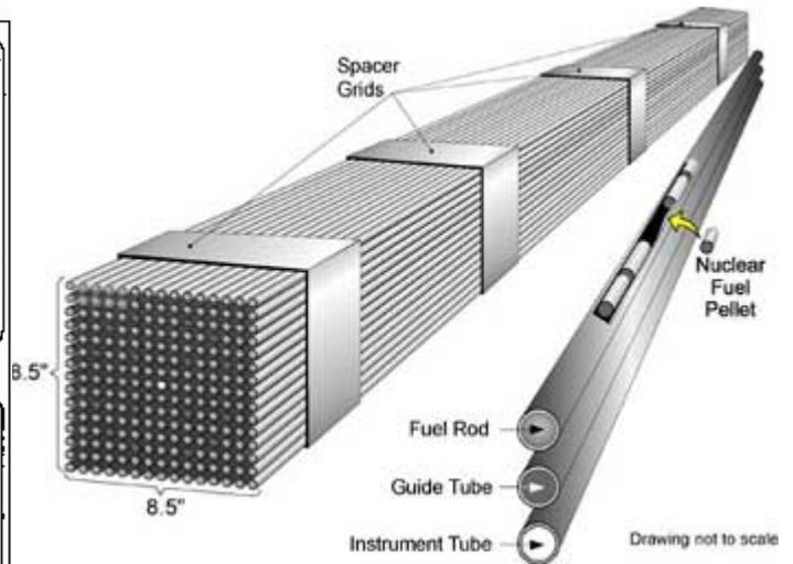
A diagram of a typical nuclear reactor fuel assembly is shown in Figure 2 (from Knief, 1990).
